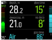
**NOTE:** Set tank size under the **Gases** menu to get the gas consumption and the gas time calculations right.
