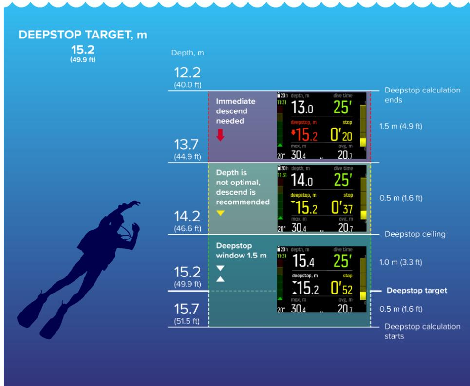
Below 20.0 m (66 ft), deepstop gets activated. In this case, as the diver ascends, the deepstop is necessary at halfway of the maximum depth, so at 15.2 m (49.9 ft).
