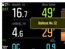
If the malfunction is rectified or the dive situation otherwise normalizes, you can switch back to a diluent using the same procedure as described above, but selecting from **CC gases**.
