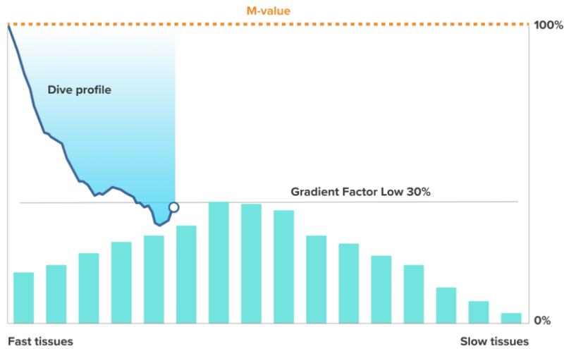
When the ascent continues, the GF moves from 30% to 70%. GF 70 indicates the amount of supersaturation allowed when you get to the surface. The lower the GF High value is, the longer shallow stop is needed in order to off-gas before surfacing. In the following illustration, GF High is set to 70% and the leading tissue compartments react to the 70% limit of M-value. At this point you can come back to the surface and finish your dive.
