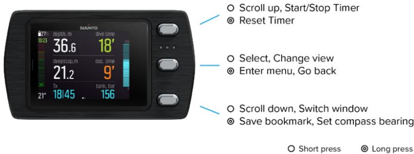
By default Suunto EON Steel Black has four main dive **modes**: **Air/Nitrox**, **Trimix**, **CCR** and **Gauge**.
