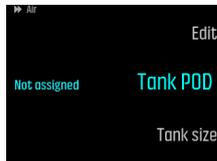
3. From the list of Tank PODs, select the one which matches the serial number of your Tank POD.
