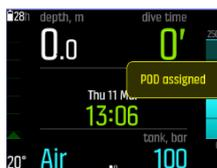
In the dive main views, only one tank pressure is shown and corresponds to the active gas. When you change gas, the displayed tank pressure changes accordingly.
