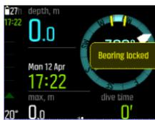
Once you have a bearing locked, the lock position is indicated on the compass rose, as shown below.
