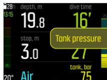
When the tank pressure drops below 50 bar (720 psi), the actual tank pressure value is indicated in red in the switch window and a mandatory alarm is triggered:
