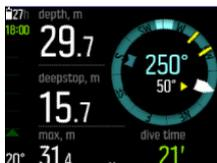
Below your heading (large number in center of compass), you also see the relative difference between your bearing and your heading. So, for instance, when you want to travel in the exact direction of your bearing, the lower number should be 0°.
