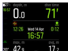
No-fly time is the minimum surface time after a dive which is recommended to wait before flying with an airplane. It is always at least 12 hours. For desaturation times shorter than 75 minutes, no-fly time is not displayed. Maximum no-fly time is 72 hours.
