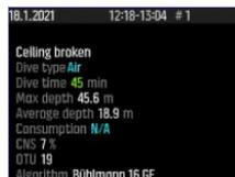
If you dive again after ceiling was broken, the new dive log has the header **Ceiling broken in previous dive**.
