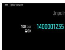
4. Make sure the Tank POD has been activated by ensuring the tank pressure reading shows on screen and POD green led is blinking.
