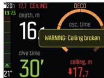
When the warning disappears, **Ceiling broken** sign becomes visible on the left side of the screen.
